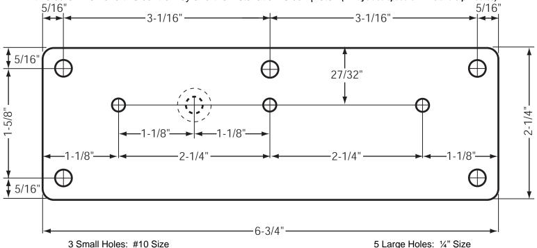
Note: The optional wiring hole and slight counter-bore (indicated by dashed circles) for the jacketed cable are only required when you have a KRD with the "-S" Switch Option.
